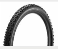
**Scorpion XC S**: Designed for riding in softer conditions, the taller centre and side knobs are widely spaced and designed to cut into soft terrain and muddy conditions when maximum grip is key.
